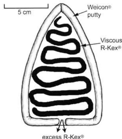
**Figure 1.** Epoxy adhesives applied to the base plate (see also Mitchell, 2000).
