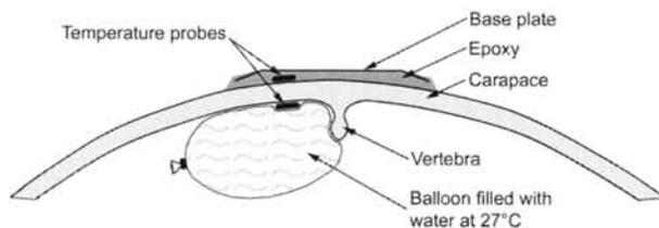
**Figure 4.** Experimental set-up for temperature measurement during exothermic epoxy curing process (cross section showing placement of temperature probes).
