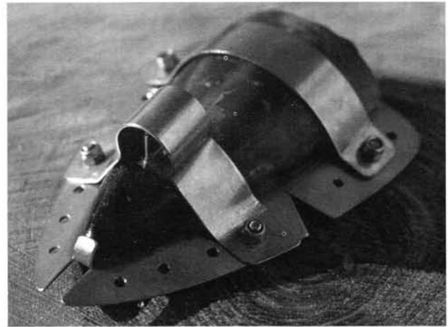
**Figure 3.** Base plate (1 mm stainless steel) and device used in 1999 field season.
